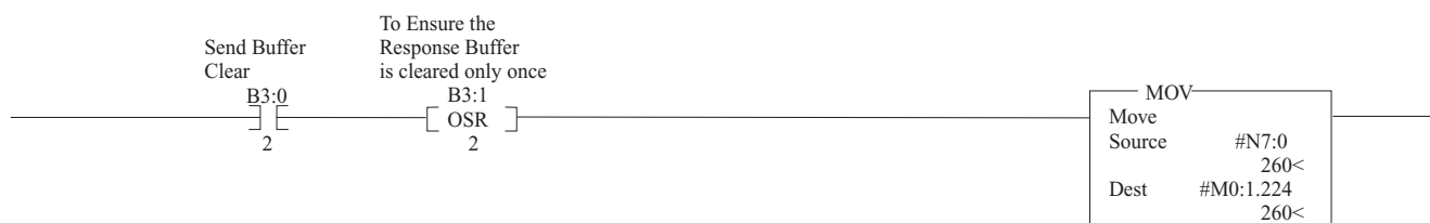
Figure C.7 Clear the DeviceNet Scanner's Response Buffer
