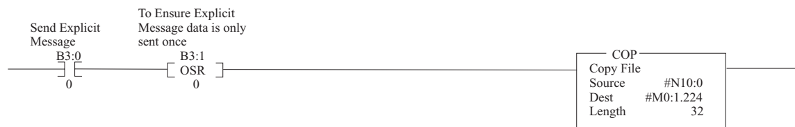
Figure C.29 Copy data from SLC Processor to DeviceNet Scanner Module
