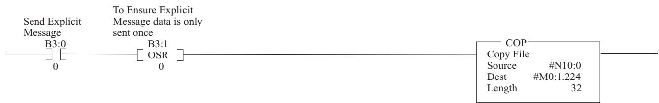
Figure C.23 Copy data from SLC Processor to DeviceNet Scanner Module
