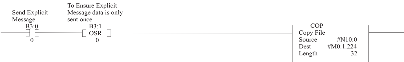
Figure C.27 Clear the DeviceNet Scanner's Response Buffer
