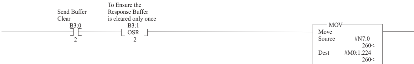
Figure C.35 Clear the DeviceNet Scanner’s Response Buffer
