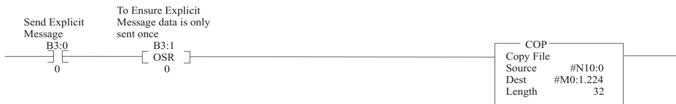
Figure C.9 Copy data from SLC Processor to DeviceNet Scanner Module
