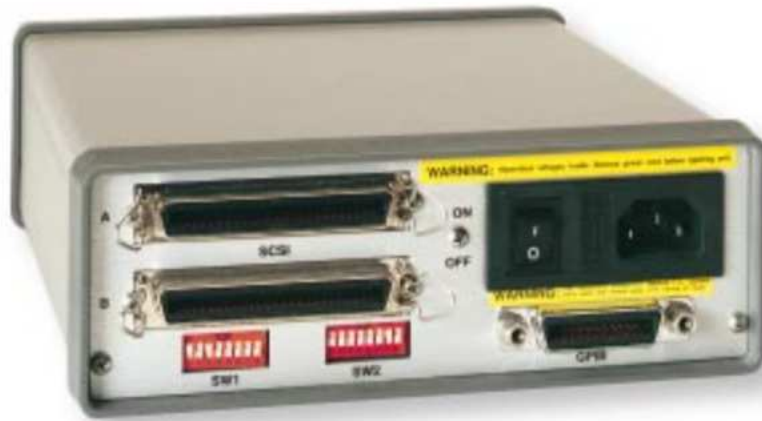
Figure 3. GPIB-SCSI-A Rear Panel
