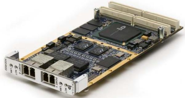
The combination of the XGE hardware based TOE performance characteristics and its programmable architecture enables the use of Gigabit Ethernet as a high performance network fabric - one that offers the ubiquity, compatibility and simplicity of standard Ethernet and the performance characteristics needed for high performance embedded systems.
