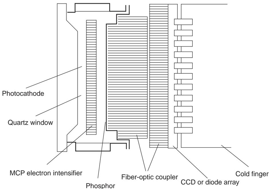
The proximity-focused MCP image intensifier is shown in Figure 1 optically coupled to a CCD or diode array with a fiber optic window. A fiber optic taper may also be used, or a lens assembly.
