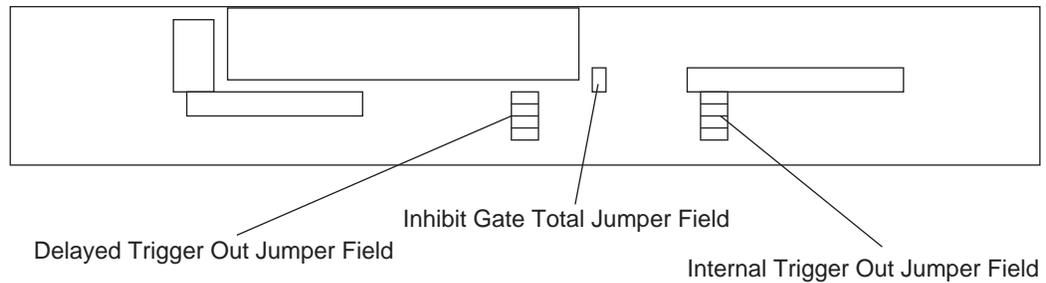
**DELAY OUT** – Located on the Front Panel Board. Normally configured for 5 V negative logic output but can be re-configured for 5 V positive logic, 15 V positive or negative logic. The JUMPERS program must be run for proper calibration following a jumper change.
