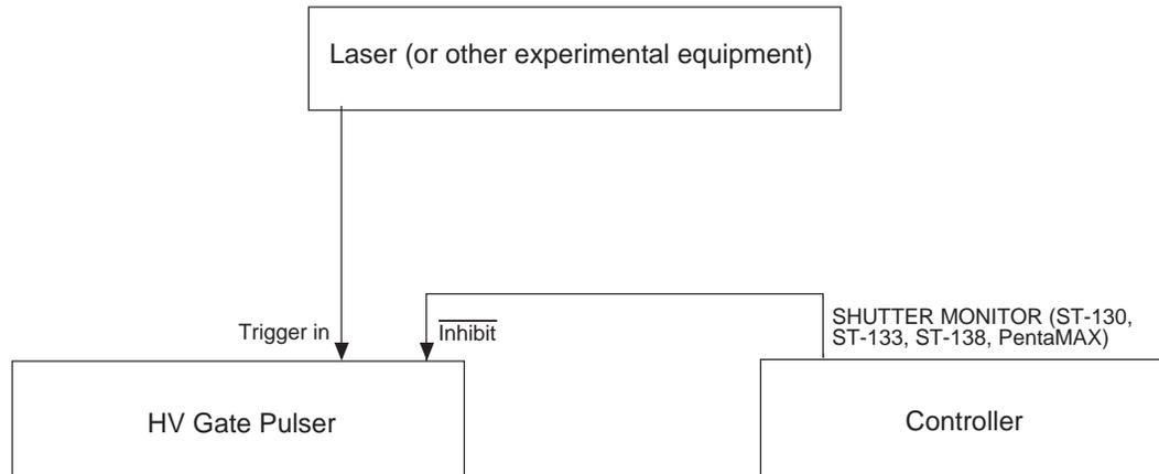
This mode of operation allows multiple laser pulses to be averaged (accumulated) on the CCD. It is usually used with high repetition rate lasers or when S/N ratio considerations require exposure of the CCD to many laser pulses before readout.
