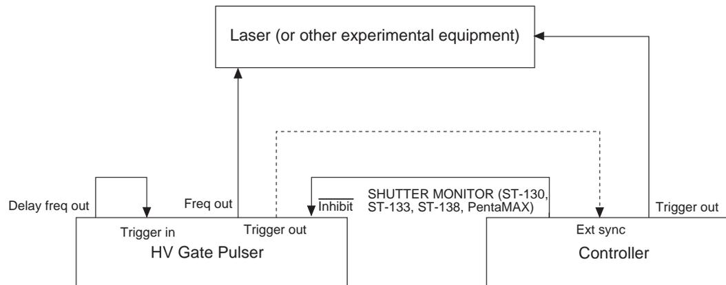
Most of the examples up to now required the laser light to be optically delayed to compensate for the delay between the laser pulse and the gate pulse. It is possible to use the internal frequency generator of the pulser to electronically delay the laser instead.
