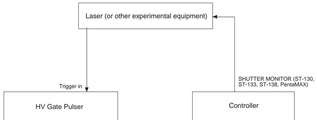
The controller is in the Freerun mode, and SHUTTER MONITOR from the rear panel of the controller is connected to the experiment. SHUTTER MONITOR goes TTL high at the beginning of each exposure cycle. The CCD readout will occur after exposure is over. Since the controller is the master, the laser is inactive and the pulser will not trigger during CCD readout.
