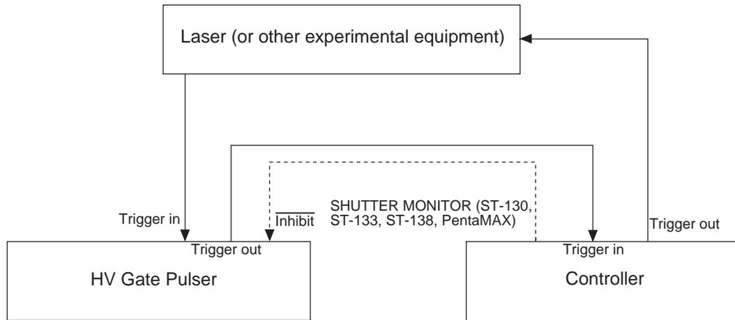
This example is used when the experiment has a long or unpredictable delay between the time it is gated and when it fires. Here, again, the controller is the master, but the CCD readout is controlled by the pulser, as in Example 1.
