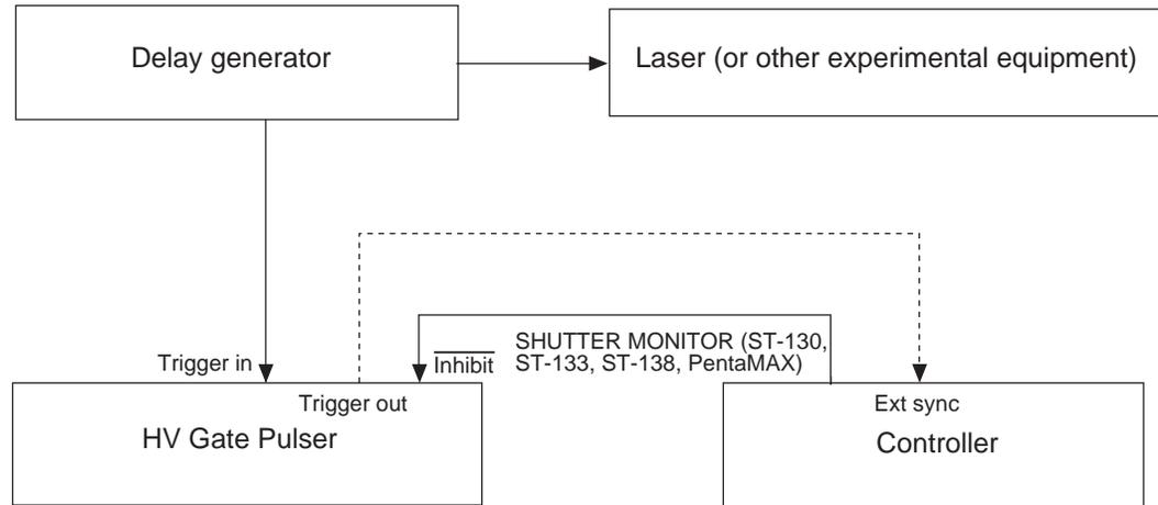
This example illustrates the use of a multichannel delay generator to control both experiment and WinView/WinSpec timing. One channel of the delay generator triggers the laser. At the appropriate time, the second channel triggers the pulser. After gating, the pulser can be used to trigger the controller, which is in the External Sync mode, or the controller can be left in the Freerun mode and SHUTTER MONITOR used to enable the pulser.
