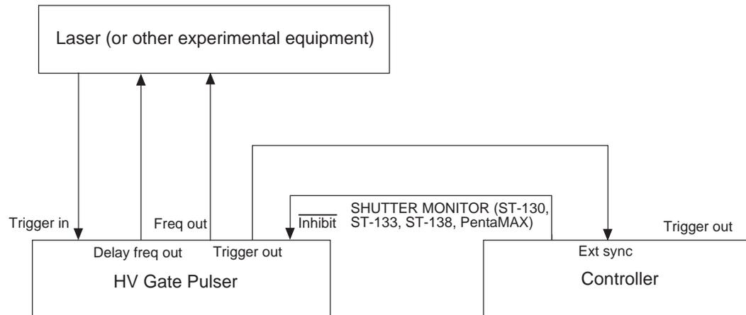
This is an example of a more complicated experimental timing sequence, requiring two system triggers. Some equipment requires a pre-trigger before being ready to fire at a second trigger. Alternatively, trigger 1 can trigger one part of an experiment; e.g., a stop flow pump, a xenon flash lamp, etc., while trigger 2 can trigger another; e.g. laser pulsing.
