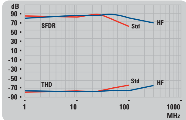
Figure 5: SFDR & THD values at 170 MS/s SR and 80% of 1 V FS are remarkably high for both the standard and HF inputs.
