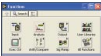
Functions Palette – Choose measurement VIs and functions to create your graphical code.
