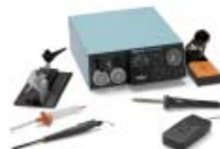
WMA 3V A single channel, analogue controlled repair station for use with compressed air or inert gas. The station is supplied with a 100 watt hot air pencil, vacuum pick up and solder paste/adhesive dispenser all able to be operated simultaneously.
