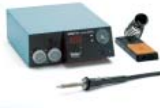
WMD 1A A single channel digitally controlled repair station with an integral pump to provide variable volume air flow and fixed value vacuum. The station is supplied with a 100 watt hot air pencil but all other Temtronic tools of compatible rating could be driven.
