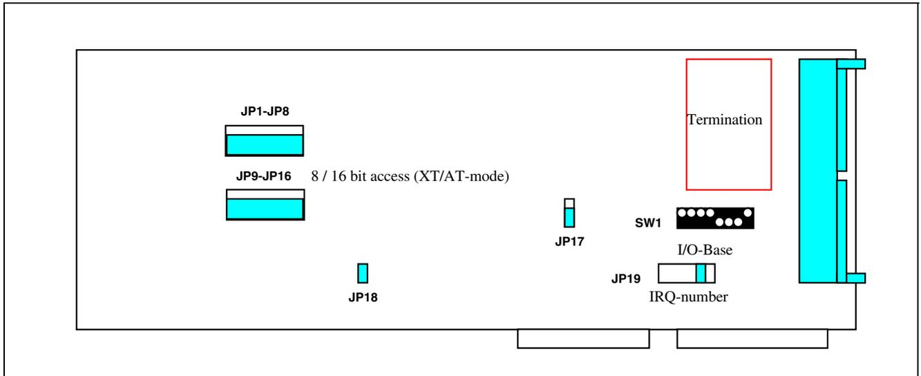
Fig. 1, PC 16 jumper and switch locations
