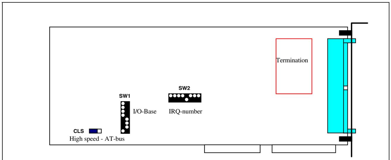
Fig. 2, PC16 - Turbo jumper and switch locations
