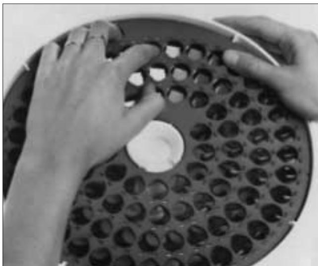
**Fig. 10.** Snapping the tube holder into place.
