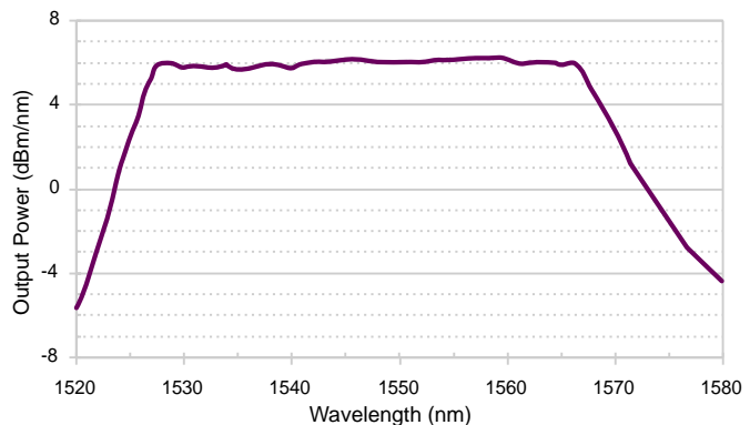
Typical power-density spectrum of the EBS-4022 Er 3+ Broadband Source, as measured with an optical spectrum analyzer using a resolution bandwidth of 1 nm.
