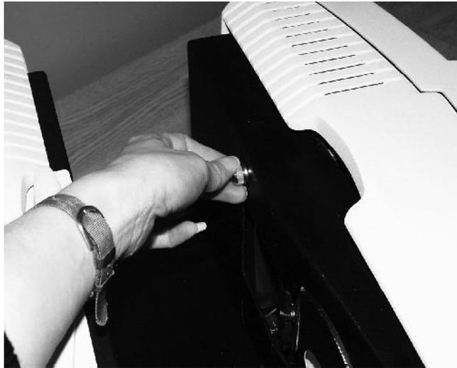
6. Remove the front cover from the instrument by sliding it forward and unplug the harness which connects the indicator lights of the front cover to the instrument.
