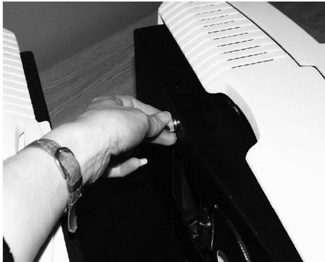
6. Remove the front cover from the instrument and unplug the harness which connects the indicator lights of the front cover to the instrument.
