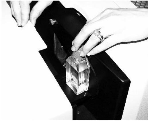
Place it as close to the **lens** as possible when measuring regular transmittance.
