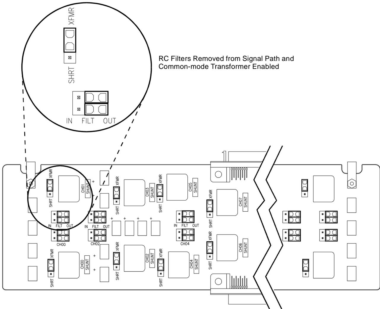
**Figure 5. Option 001 Three-Wire Cable Configuration**
