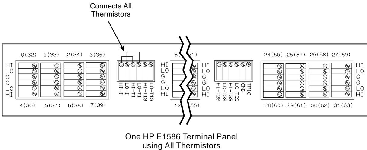
Figure 3. Connecting Three Thermistors on a Single Panel
