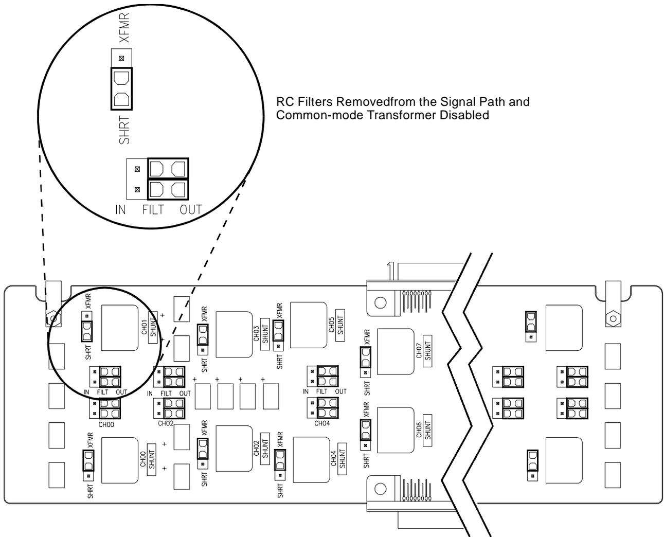
RC Filters Removed from the Signal Path and Common-mode Transformer Disabled
