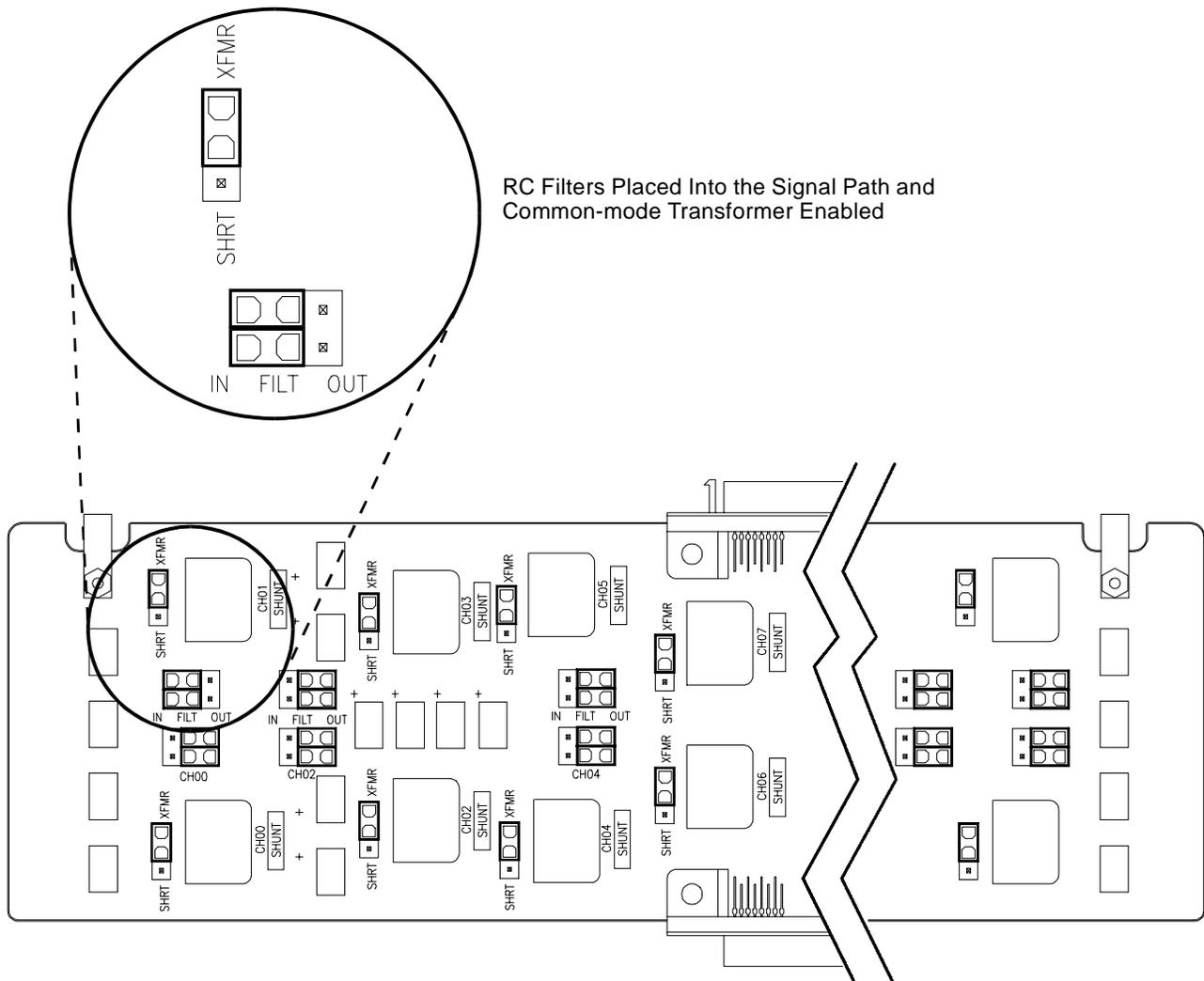
**Figure 6. Option 001 Two-Wire Cable Configuration**
