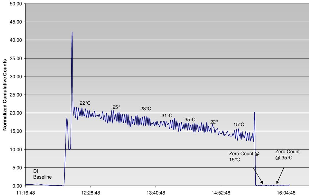
Figure 3. Particle concentrations at various casing temperatures. This demonstrates the independence of true particle counts and temperature. The decreasing counts are caused by the plumbing becoming clearer.
