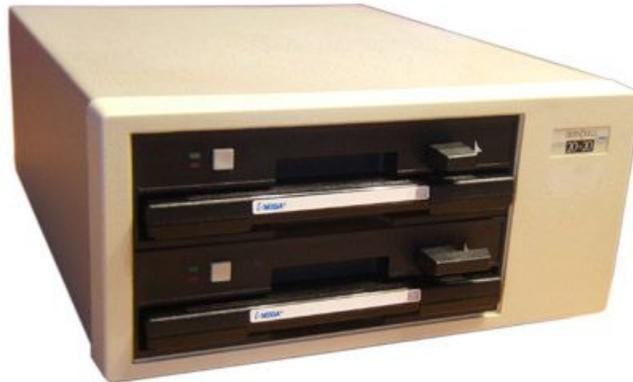
Before Iomega became known for Zip drives it produced a very high quality removable cartridge storage system known as the Bernoulli Box. At a time when floppy drives held only 360KB or 1.44MB of data and hard drives only held 10 to 30MB of data the Bernoulli Box offered data storage limited only by the amount of removable cartridges you wanted to own. The cartridges were very robust and withstood abuse well, making them a pricey but ideal format for large scale removable storage.
