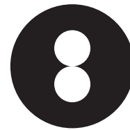
Fig. 3 Front view of common end of a bifurcated liquid light guide. The end does not merge into a single circular core.
