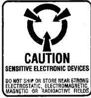
The board utilizes static sensitive components and should only be handled at a static-safe workstation.
