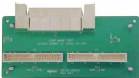
Figure 1-5 Connecting the Loop Back Board to the N5102A Module
