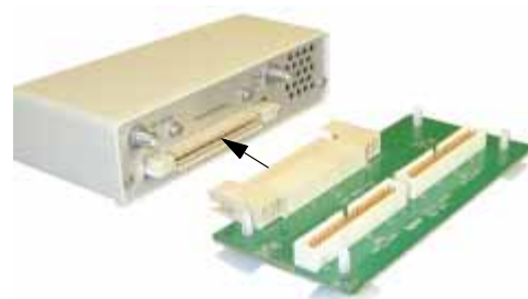
Figure 1-5 Connecting the Loop Back Board to the N5102A Module
