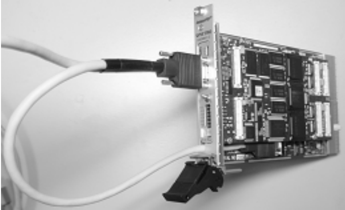
Figure 2.8 Connect the 15 pin mDSUB to the PBTM-515 front panel
