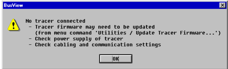
Figure 5.1 Warning message indicating that BusView was not able to connect to the PBT(X)-515
