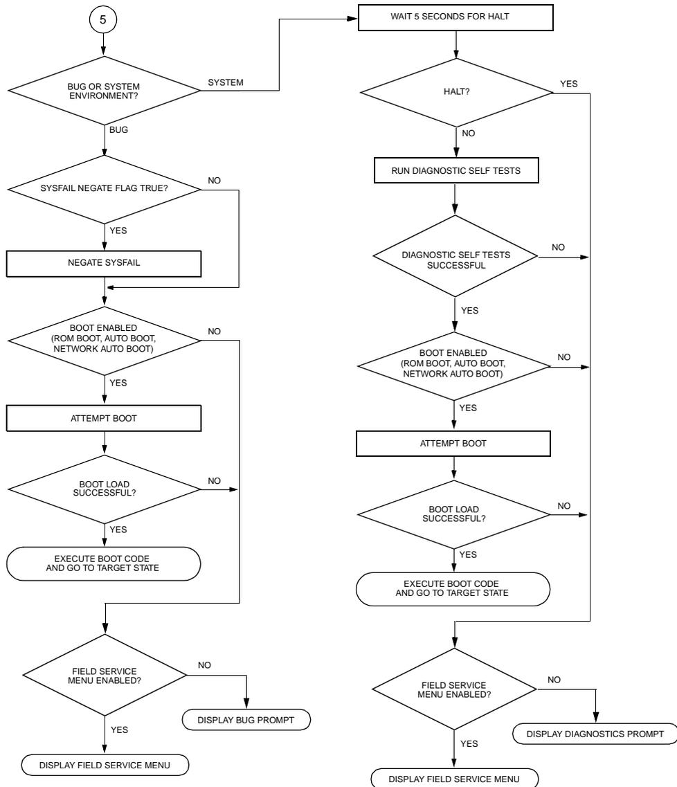
**Figure 1-1. 177Bug Start-up Flow (Sheet 3 of 3)**
