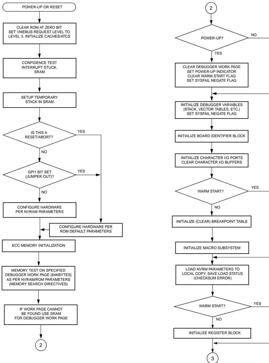
Figure 1-1. 177Bug Start-up Flow (Sheet 1 of 3)
