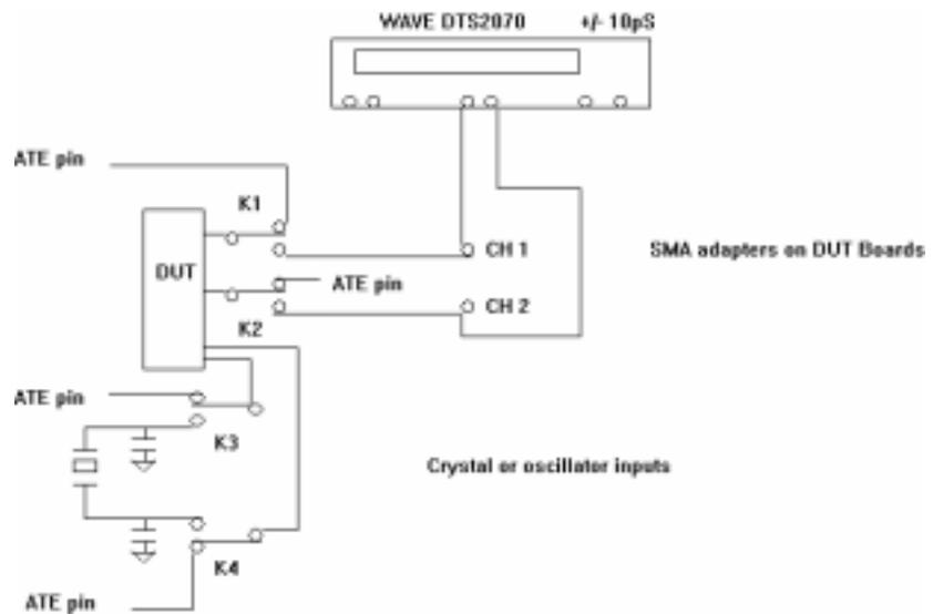
**Diagram no. 1 DUT Board Relay Matrix.**
