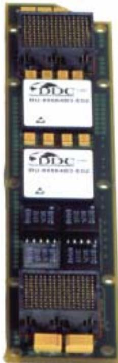
Figure 10: Interface Personality Module with MIL-STD-1553
