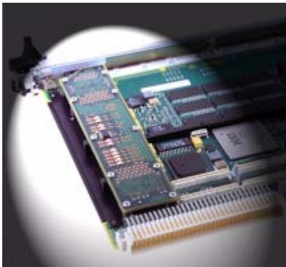
Figure 5: Interface Personality Module (IPM) Adds Flexibility
