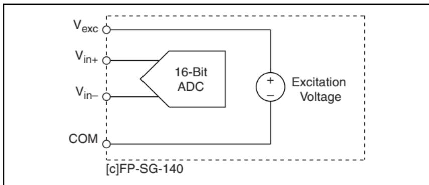
**Figure 3.** [c]FP-SG-140 Input Circuit
