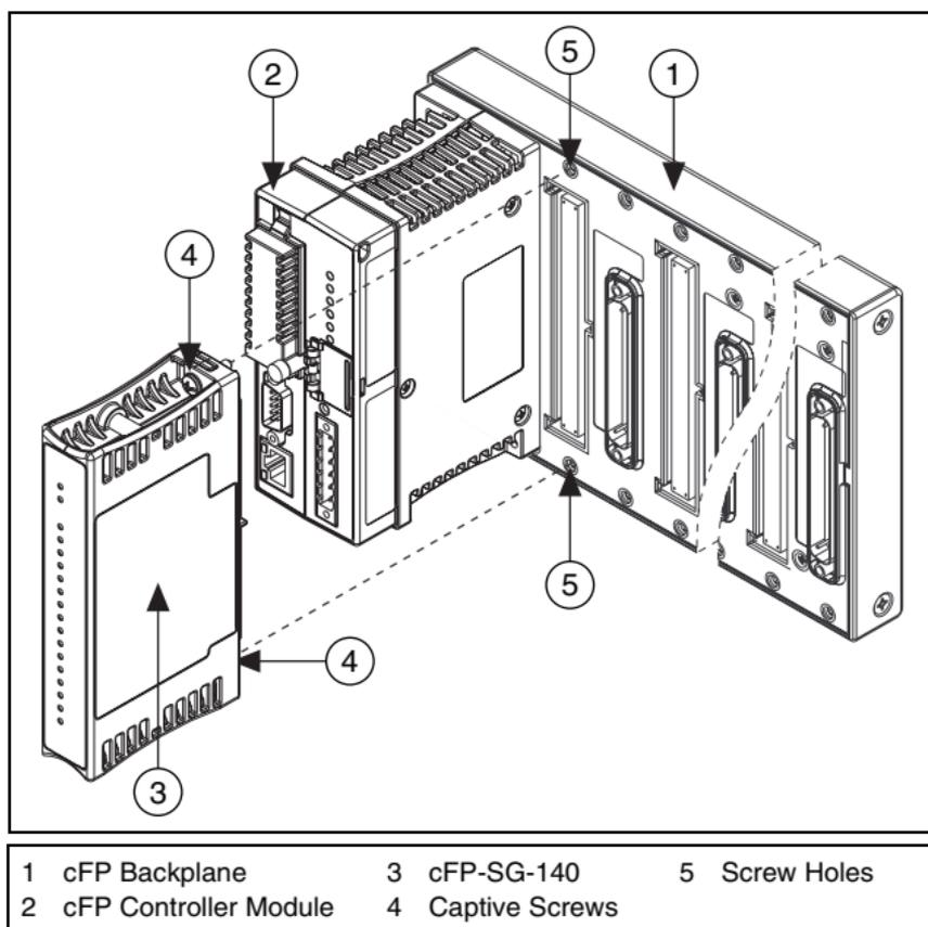
**Figure 2.** Installing the cFP-SG-140
