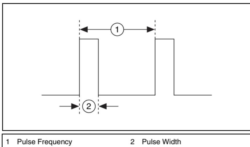
**Figure 8.** Pulse Width and Pulse Frequency
