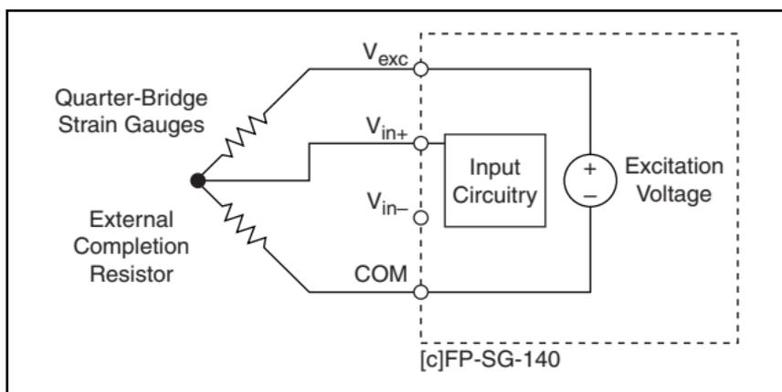
**Figure 6.** Connecting a Quarter-Bridge Strain Gauge to One Channel
