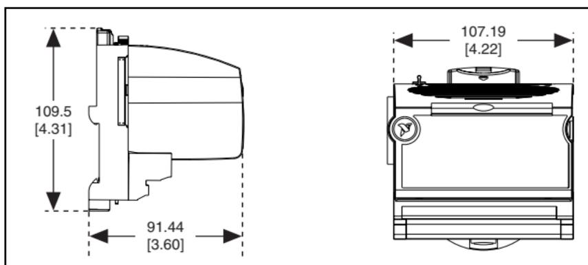
**Figure 9.** FP-SG-140 Mechanical Dimensions
