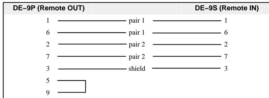
**Figure 6-1 InterBus-S Remote Cable**
