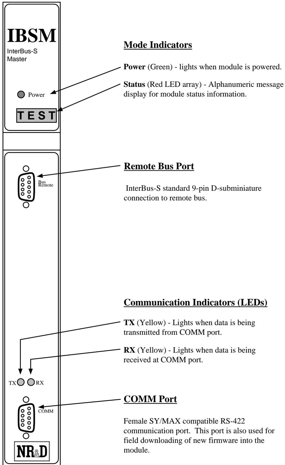
Figure 1-1 IBSM Front Panel
