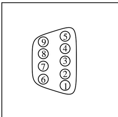
Figure 5-1 SY/MAX RS-422 Connector Pinout
