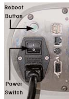
Electrical Connection Panel
