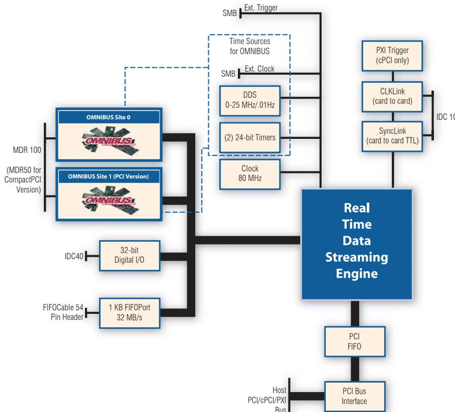
ChicoPlus is a common platform baseboard providing the data moving functions and numerous generic peripherals while the OMNIBUS mezzanine cards of your choice will provide the type of analog channels specific to YOUR application.
