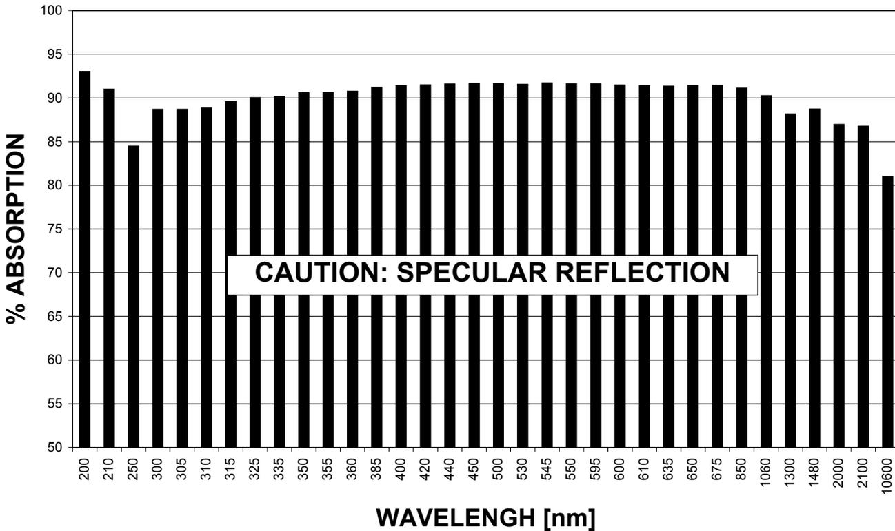
**NOTE:** Please exercise caution when using HD detectors. They exhibit spectral reflection of between 7% and 33%, of the input power, back out of the aperture. Please refer to figure above to determine the reflectance for the wavelength you are measuring. These detectors should be treated as a partial mirror or any other type of reflective optic and the appropriate caution level observed, especially in the CO<sub>2</sub> wavelength.
