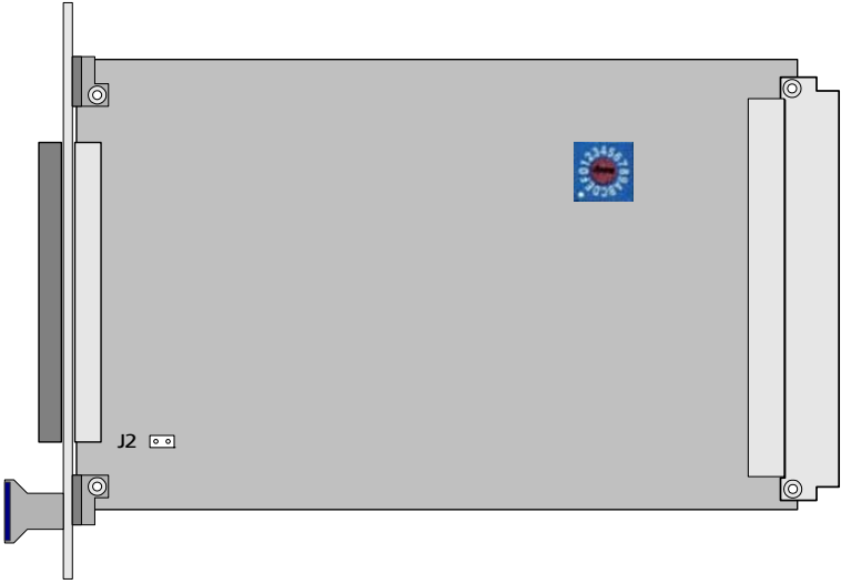
Fig. 2-3 Position of the jumper and the hex switch (board Rev. 1.1, component side)
