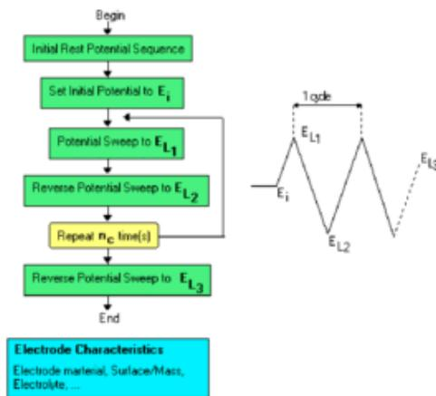
General flow-diagram for Cyclic Voltammetry
