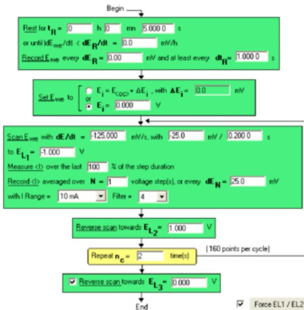
Cyclic Voltammetry detailed flow diagram
