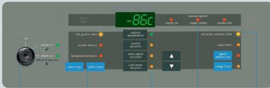
**Setpoint security system with key-operated switch**
