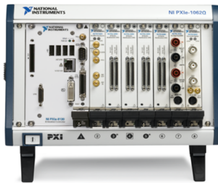
Figure 1. This NI PXIe-8130 controls an 8-slot PXI Express modular instrument and data acquisition system.
