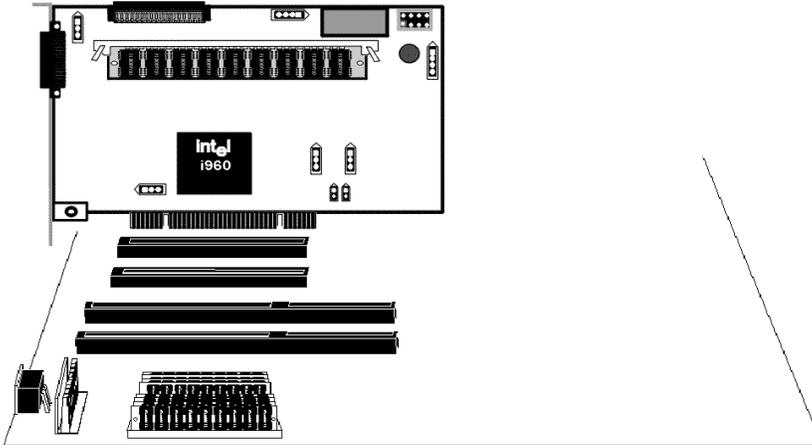
Screw the bracket to the computer frame.
