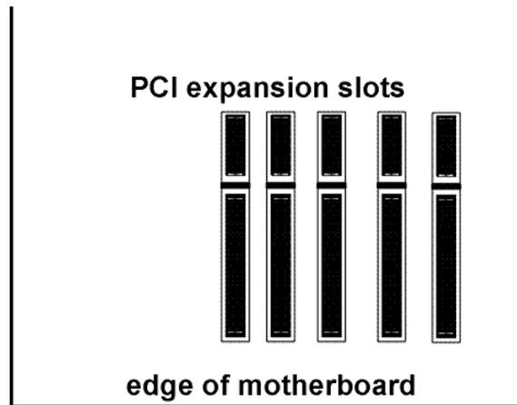
Insert the MegaRAID Express Plus card in a PCI slot as shown below:
