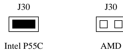
Figure 3-2. J30: CPU Voltage Settings
