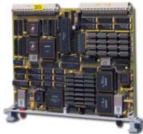
The local SRAM provides fast Read access times to stored data. Writes are stored in local SRAM and broadcast over a high-speed fiber-optic data path to other Reflective Memory nodes. The transfer of data between nodes is software transparent, so no I/O overhead is required. Transmit and Receive FIFOs buffer data during peak data rates to optimize CPU and bus performance to maintain high data throughput.
