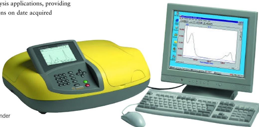
Figure 15. Ultrospec 3100 *pro* under PC control using SWIFT II.
