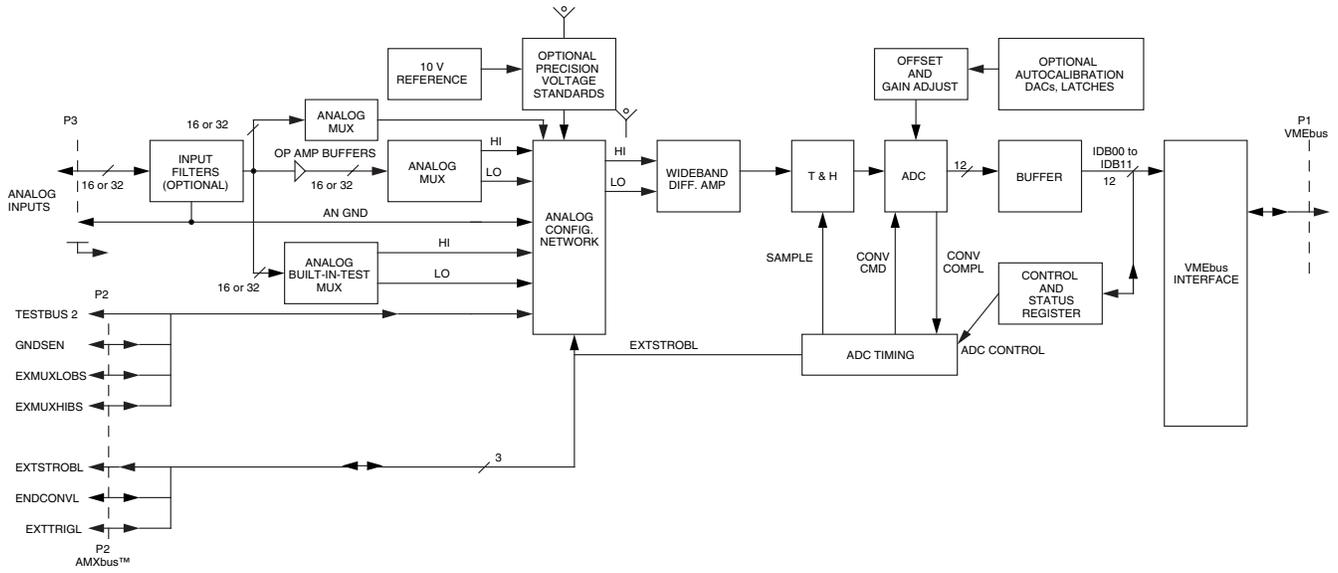
**Figure 1. VMIVME-3101A Functional Block Diagram**
