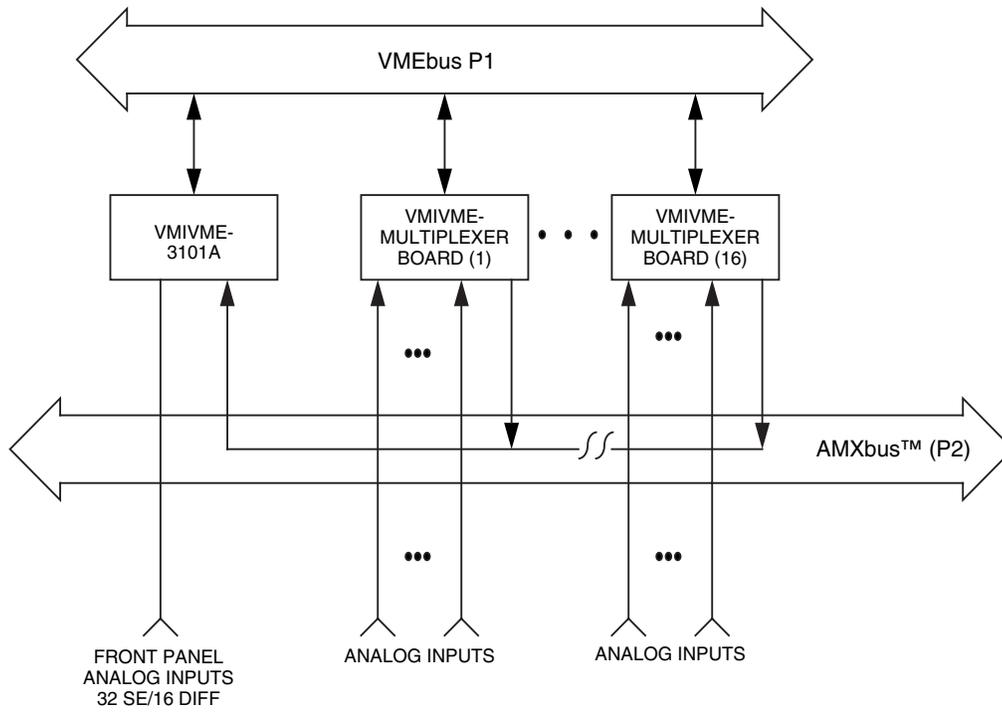
Figure 5. VMIVME-3101A Typical Configuration with Multiplexer Expansion
