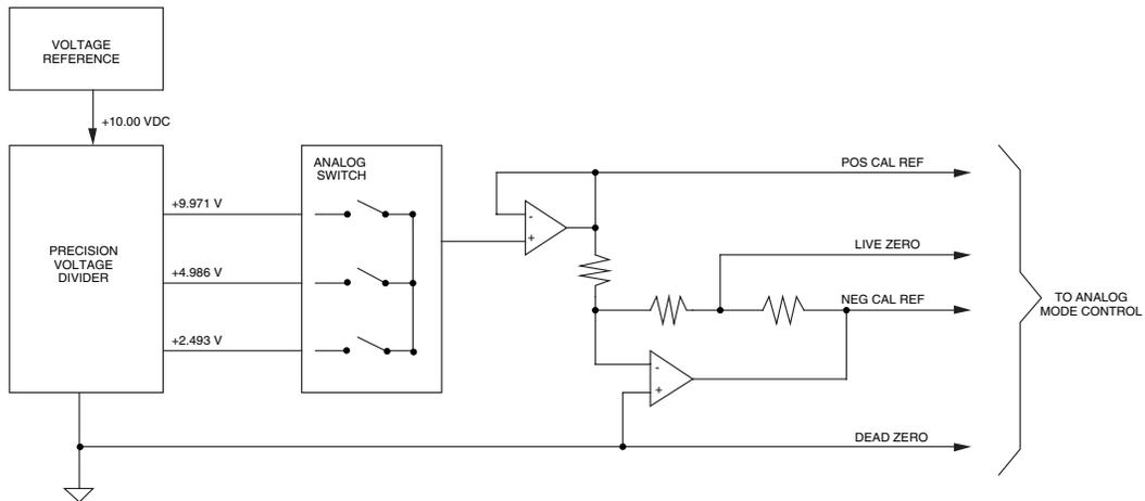
**Figure 2. VMIVME-3101A Precision Voltage Standards Network**
