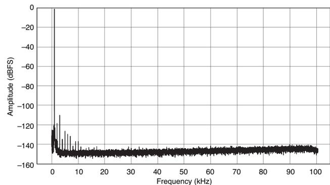
Figure 1. FFT of -1 dBFS, 1 kHz Tone Acquired at 204.8 kS/s and 0 dB Gain Using the NI PXI-4498 (65,536 Samples with 10 RMS Averages Using the 7-Term Blackman-Harris Window)
