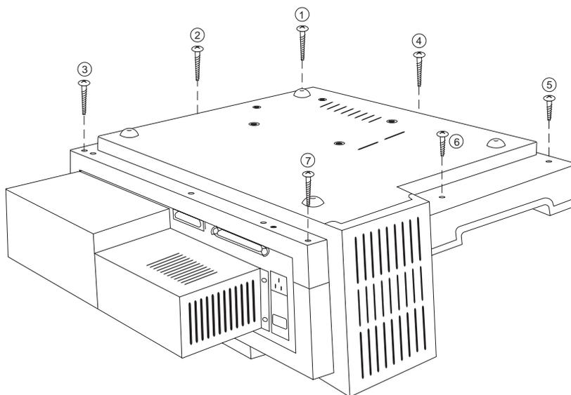
*Figure 8: Underside of the Microplate Reader. This illustration shows the location of the seven screws that need to be removed before separating the top and bottom halves of the casing. Note: depending on the model you have, the back of the plate reader may not look exactly like this.*
