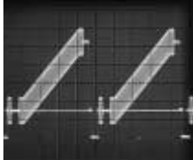
Horizontal line TV signal
