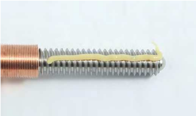
Fig. 4.1 Greasing the Leadscrew
