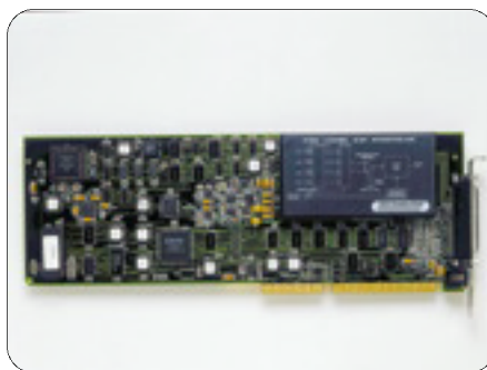
DT2802 Series 24-Bit Chromatography Boards for the ISA Bus
