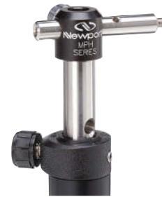
The MPH-0.5C (M-MPH-0.5C) is cross-bored to allow horizontal post mounting.
