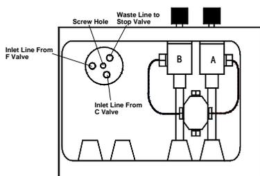
After assembling the three tubes into the pressure plate the assembly can be fixed to the cell block from inside the sample handling unit water bath. (See diagram to left.) This is most easily done by removing the “C” and “F” valves to allow good access to the rear of the cell block.
