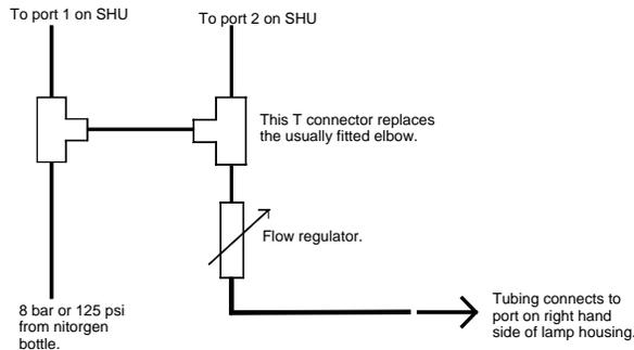
If nitrogen is being used as the main drive gas supply then the elbow on the 'h' connector used to connect the gas supply to the back of the sample handling unit can be replaced with the supplied flow regulator assembly as shown in the diagram to the left. The tubing on the outlet of the flow regulator should be connected to the purge inlet on the right hand side of
