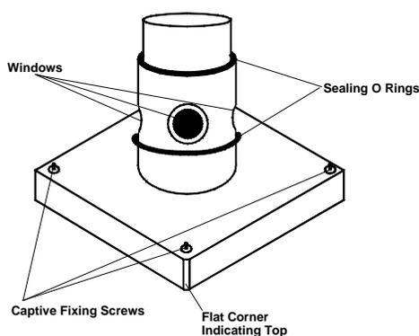
Cells are mounted in a cartridge, shown in the diagram to the left. To change the cartridge, first remove the light guide from the cell block. Then drain the thermostat water from around the drive syringes and remove the water bath front plate. Next, loosen the tubing pressure plate that forces the flow tubing onto the cell. (See section 3.23 for more information regarding the pressure plate.) Finally undo the four captive fixing screws and remove the cell cartridge.
