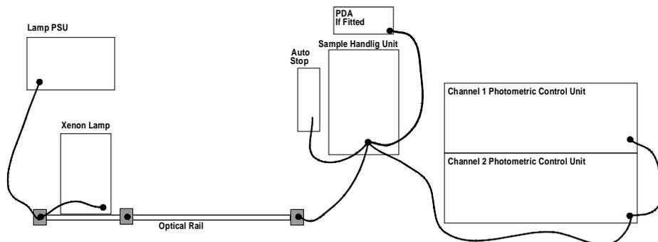
**Rear View of System Showing Grounding Connections**
