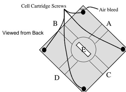
The fluorimetric port, E, is at the back of the cell block and the Emission Photomultiplier (high sensitivity) should be mounted using the rubber light seal, finger screws and nylon washers provided. When measuring fluorescence the excitation light guide should be connected to the D port to give the best illumination and lowest inner filter effect.
