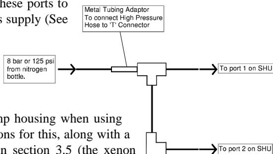
for supplying nitrogen to the lamp housing when using ozone producing lamps. Instructions for this, along with a connection diagram are shown in section 3.5 (the xenon lamp section)
