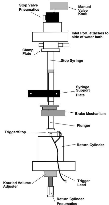
The Auto Stop mechanism, shown to the left, is fixed to the front left hand side of the Sample Handling Unit. The valve and the return cylinder are both controlled from the workstation, although both can be operated manually as long as the pneumatic drive pressure has been removed, (when flushing the system, for instance). The three pneumatic inlets are connected to three solenoids inside the Sample Handling Unit.
