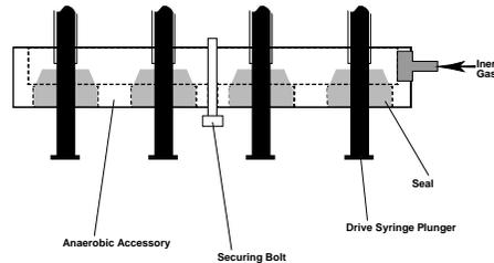
The second opportunity for oxygen contamination is from the flow tubing. Current system are shipped with PEEK tubing and PEEK drive valves as standard. This minimises the danger of oxygen contamination from the tubing and the valves.
