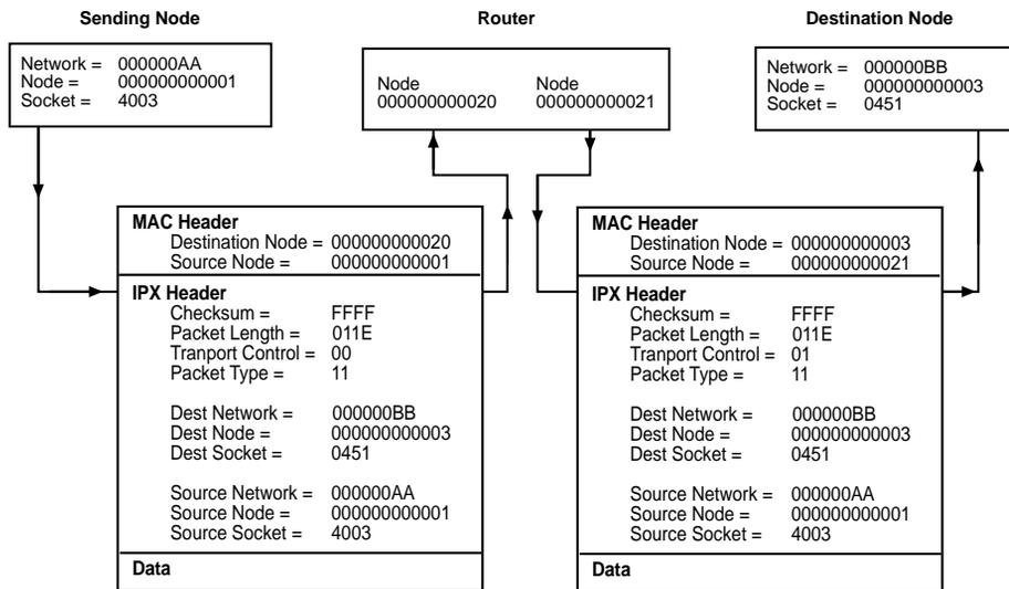
Figure 5-3 IPX Packet Routing
