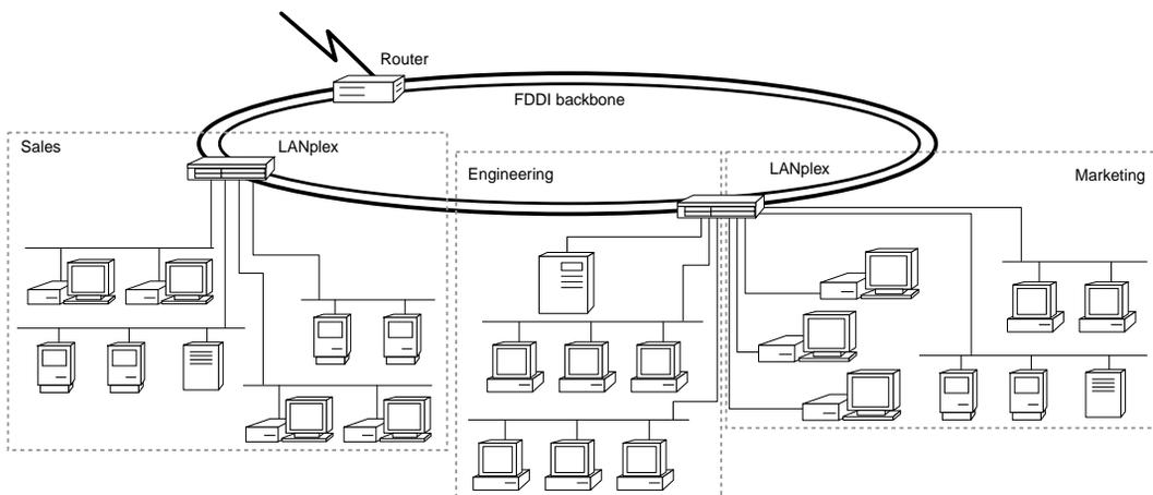
**Figure 3-2** Subnetted Architecture with LANplex Switching Hubs
