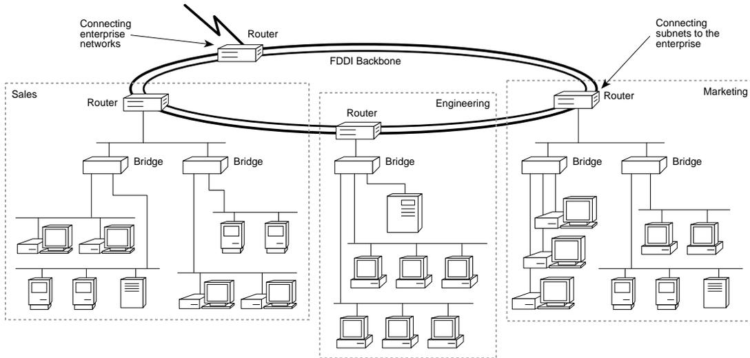
**Figure 3-1** Traditional Architecture of a Routed Network
