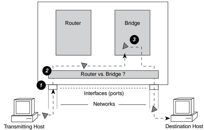
**Figure 3-4** Bridging in the Traditional Bridging/Routing Model
