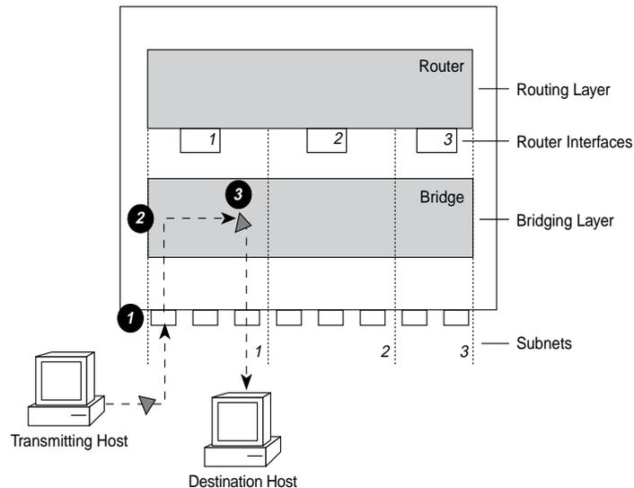
**Figure 3-6** Bridging and the LANplex Bridging/Routing Model
