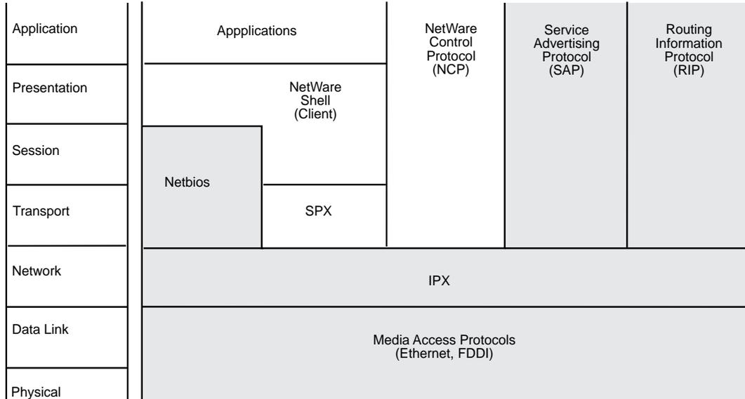
**Figure 5-1** NetWare Protocols and the OSI Reference Model
