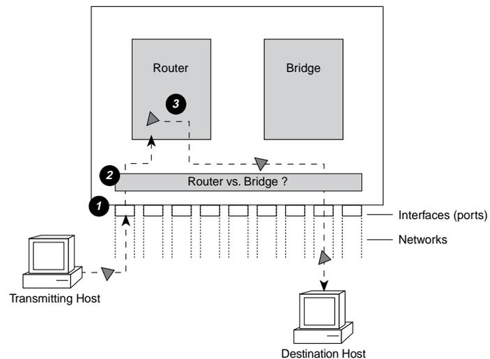
**Figure 3-5** Routing in the Traditional Bridging/Routing Model
