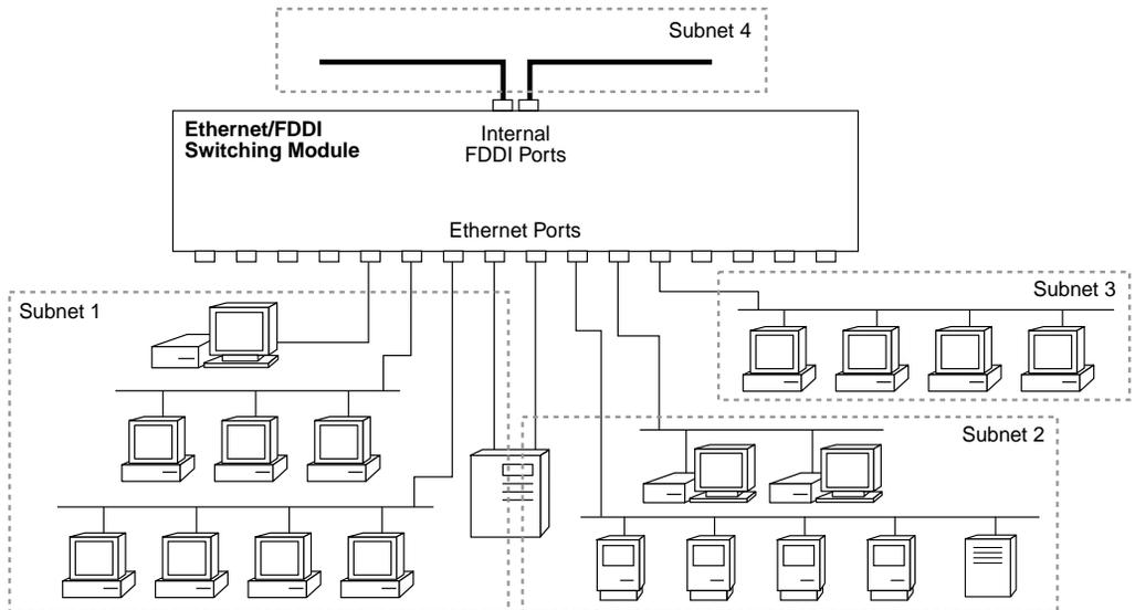
**Figure 3-3** Multiple Ports per Subnets with the EFSM
