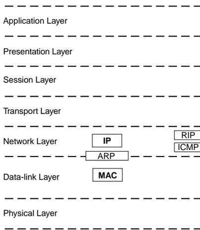
**Figure 4-1** OSI Reference Model and IP Routing
