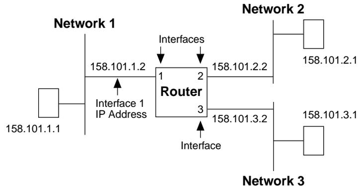
Figure 4-4 Router Interfaces
