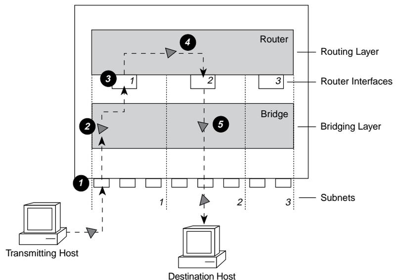
**Figure 3-7** Routing in the LANplex Bridging/Routing Model
