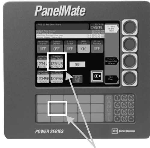
On Keypad units, pressing on the "TouchPanel" activates the template in the corresponding area of the display.
