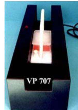
cm wide by 64 cm long and 16 cm tall. This stirrer will stir one deep well microplate at a time at up to 100 lifts/minute.
