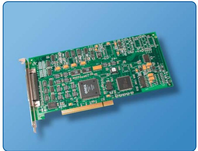
**Figure 1. The DT300 Series is a family of low-cost, multifunction PCI bus-mastering boards.**
