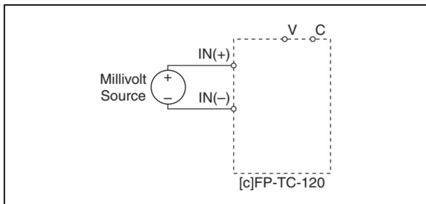
**Figure 4.** Connecting a Millivolt Source to the [c]FP-TC-120
