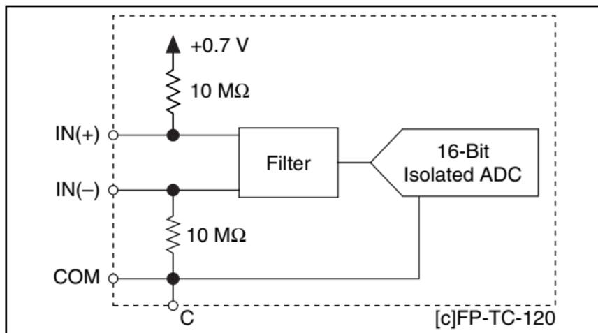
**Figure 3.** [c]FP-TC-120 Analog Input Circuitry on One Channel
