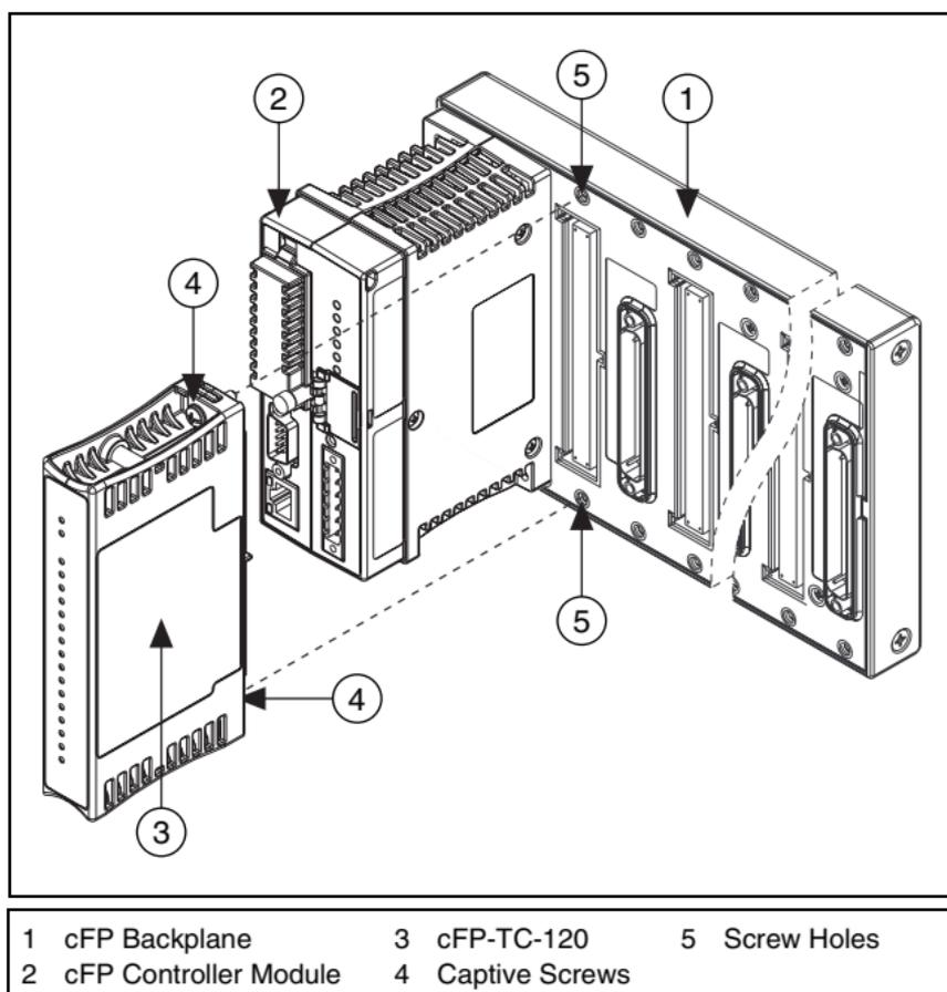
**Figure 2.** Installing the cFP-TC-120
