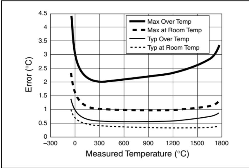
**Figure 6.** Type R and S Errors
