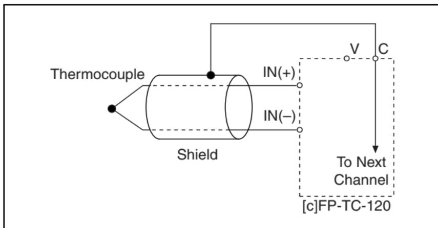
**Figure 5.** Connecting a Shielded Thermocouple to the [c]FP-TC-120
