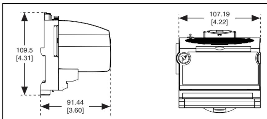
**Figure 10.** FP-TC-120 Mechanical Dimensions
