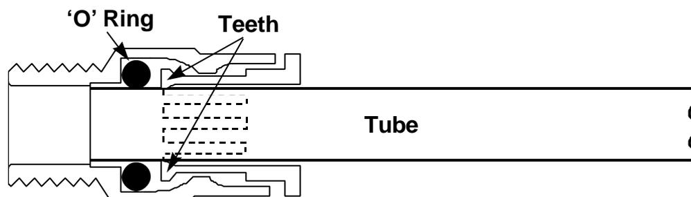
The above diagram shows a cross section of a nylon tube in a Quick-Fit Connector. The teeth (indicated) grip the tube when it is pushed into the connector. THIS DOES NOT SEAL THE TUBE IN THE CONNECTOR. THE TUBE MUST BE PUSHED THROUGH THE 'O' RING TO MAKE IT AIR TIGHT, A TOTAL DISTANCE OF 15-16MM.
