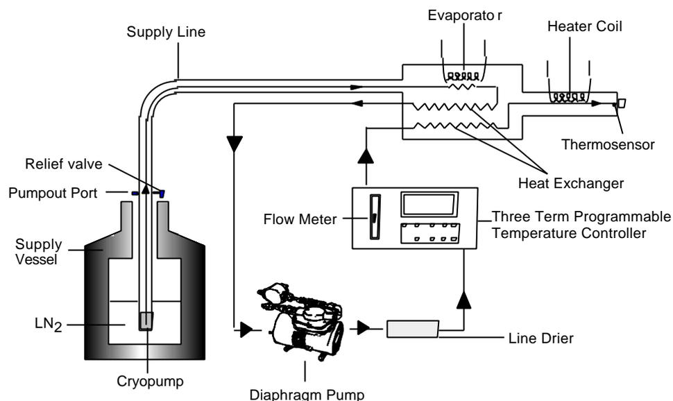
Liquid nitrogen is drawn up by the action of the Diaphragm Pump from an unpressurised Supply Vessel, through a flexible vacuum insulated Supply Line, into the Cryostream Cooler Coldhead. The Supply Vessel can be any convenient container of liquid nitrogen such as a conventional metal Dewar. Please note that the Dewar vessel is *not* sealed. This is a unique feature to Cryostream Cooler.
