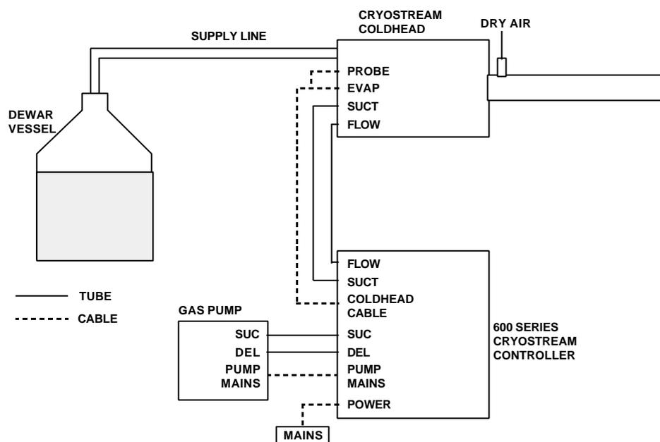
The diagram above illustrates all the connections that have to be made, full lines denote 6mm (outside diameter) nylon tubing and the dotted lines denote electrical cables. Connections are generally labelled equivalently at each end. (The table below outlines which tubes go in which connectors). The Nylon Tubeset provided with the Cryostream Cooler consists of five 6mm (outside diameter) nylon tubes:
