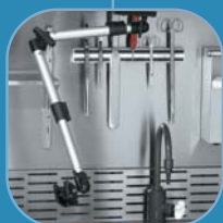
Shandon Gross-Star Workstation camera bracket and magnetic instrument bar.
