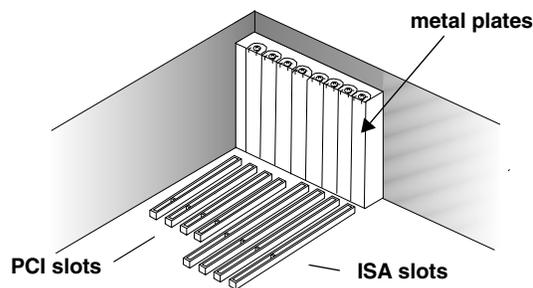
Figure 1. Locating a PCI slot
