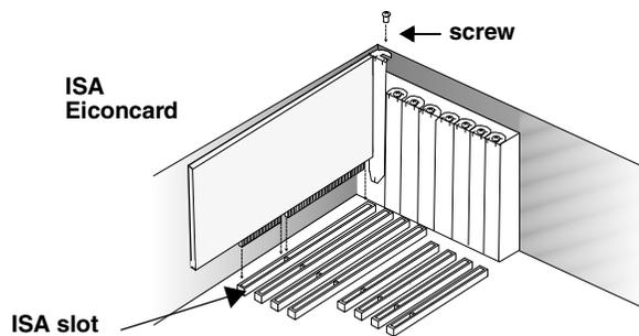
Figure 2. Inserting the Eiconcard S5x.
