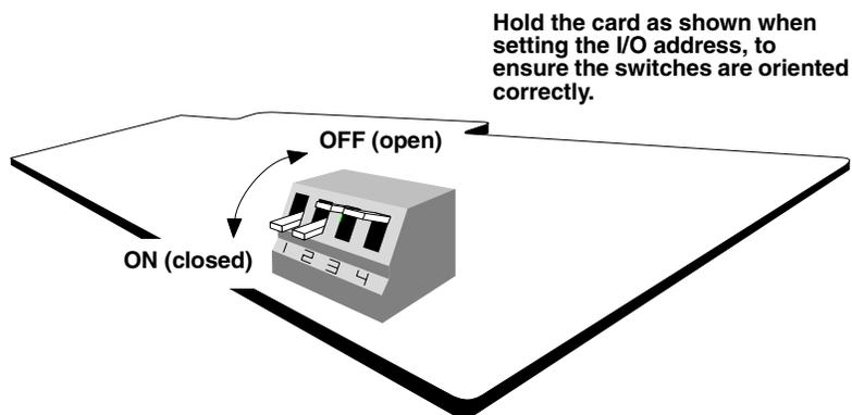
*Figure 12. I/O Address Switch*
