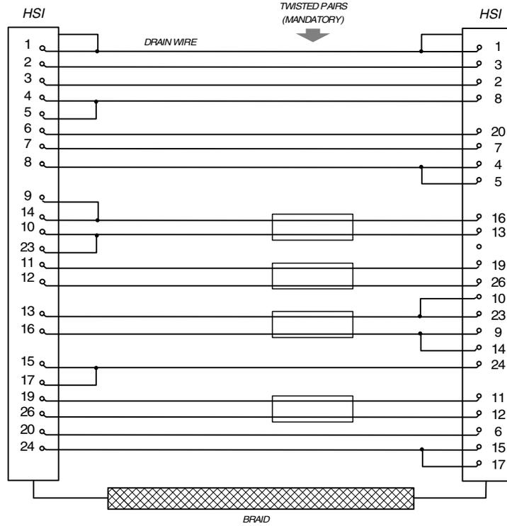
Figure 11. HSI Null-Modem Conversion Cable (300-033)
