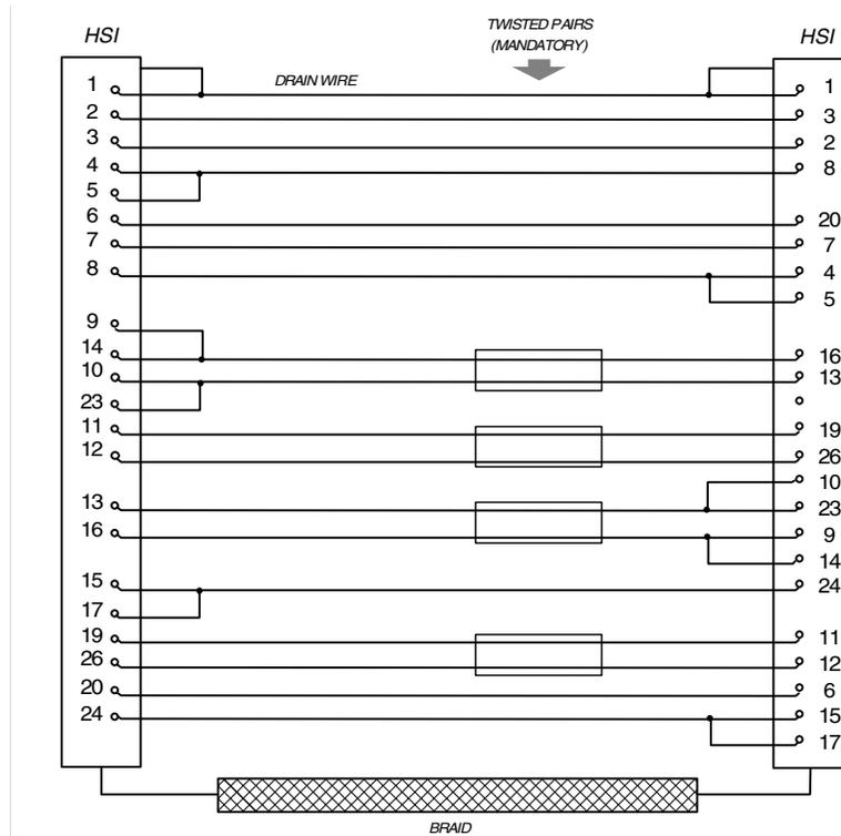
Figure 8. HSI V.24/V.35 Null-Modem Cable (300-031)
