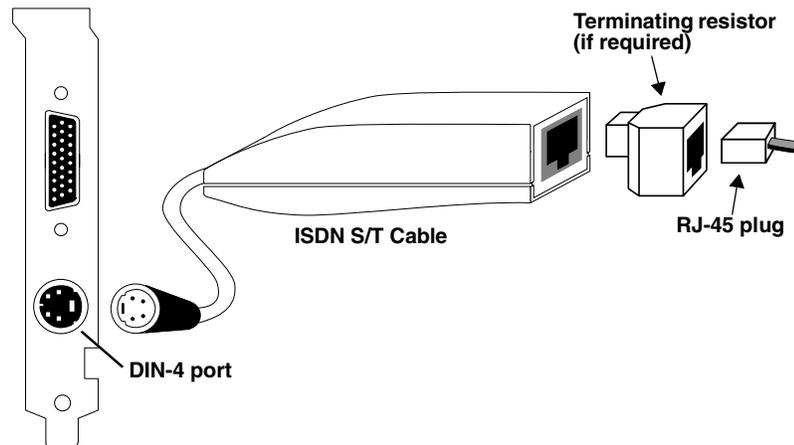
Figure 4. Connecting the ISDN S/T Cable
